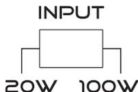
The **HLC 4 EVO** has an input power selector to adapt as many different radios and sound systems as possible. For standard OEM-headunits select „20W“. When using the **HLC 4 EVO** with a amplified sound system with more than 20W output power select „100W“
