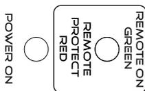
The **HLC 4 EVO** has a multi-level status display. If the **HLC 4 EVO** has recognized a signal, the "POWER ON" LED switches on. As soon as the remote output is activated, the "REMOTE ON" LED switches green, in the event of an error the LED switches red.
