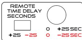
The **HLC 4 EVO** features an adjustable ON / OFF remote delay . Switch „REMOTE TIME DELAY SECONDS“ to „-25“ for turn-on delay or to „+25“ for turn-off delay. The delay time is adjusted by the potentiometer between 0 and 25 seconds.
