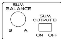
The **HLC 4 EVO** has a summation function. This adds up the inputs A + B and generates a mixed signal on output B (sum). To do this, the **SUM** switch must be set to "ON" . With the potentiometer **BALANCE** mixing ratio between Channel „A“ and „B“ can be set.
