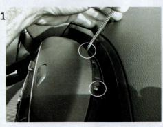
1 Remove the plug over the original radio and save the screws.
