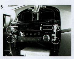
5 Remove the original radio from its position by unscrewing the screws.
