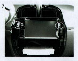
7 Place and fix with the supplied screws the aftermarket head-unit to the dashboard.
