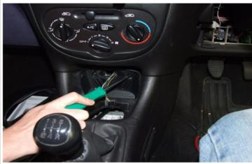
Feed the hazard wires through the relocation front panel.
