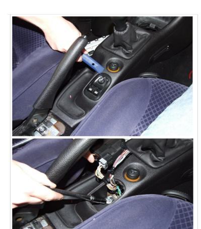
Unwrap hazard switch wiring to leave enough to allow the wire to reach the ashtray.
