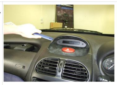
Remove screws holding display and remove display. Disconnect wiring and push wiring out the way.
