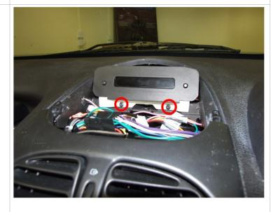
Cut plastic along red lines following the shape of the plastic sides, be careful not to cut any wires. After cutting the plastic can be removed by a gentle side to side twist to break the melted plastic joint.
