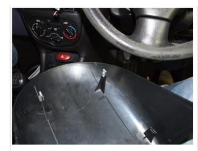
Locate the hood front clips into the stereo side brackets. Once the clips are in place, push down to clip the hood into place.
