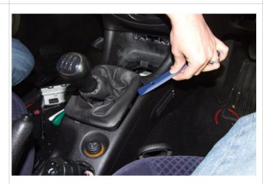
Remove the ashtray lighting wire by pushing downwards
