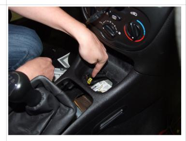
Remove Centre console front trim cover and screws these screws will be used to hold the new 2Din Stereo brackets at their rear mount point.
