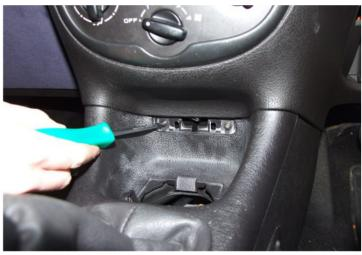
Remove window control switch panel to reveal a 10mm nut holding the centre console in place.
