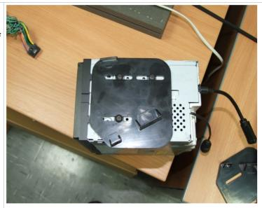
Connect all cables to the back of the stereo prior to installing in car as they are awkward to get to afterwards. Using the screws previously removed from the dash re fit them over the new brackets (front holes).
