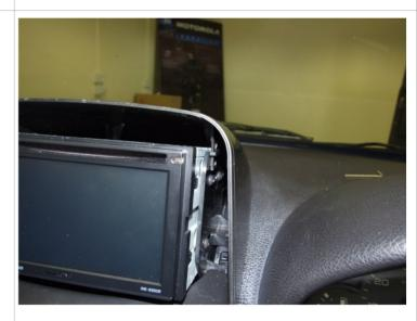
The front part of the hood has a trim which may or may not be needed depending on the stereo choice. Fitting the trim is just a case of pushing it onto the lip of the front panel taking note there is a rounded corner and a square corner
