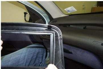
The hood front is simply clipped into place on the front of the hood back. Installation is now complete.
