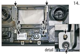
14. Attach air condition control unit to center cosole. Put metal frames over air condition control unit - attach 2-DIN facia plate
