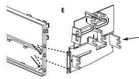
Remove all mounting tabs from the left and right side brackets. File flush with outside edge of mounting brackets
