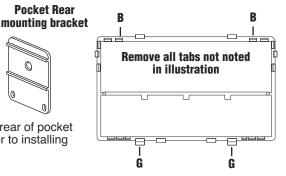
NOTE: Attach rear support bracket to rear of pocket using (1) screw, included just prior to installing radio/kit assembly into dash.
