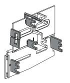
Remove all shaded tabs shown above on left and right brackets. (Left bracket not shown)
