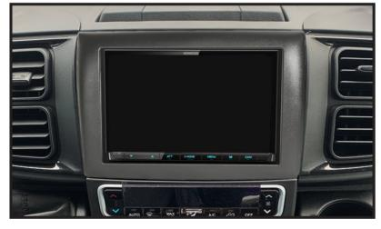
With the cage in place, and the head unit connected correctly, proceed to slot the radio into the dashboard until it clips into place. Carry on to finish the installation by placing the trim around the head unit and re-assembling the dashboard in revere order.
