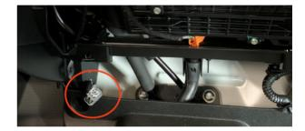
5. Connect the power/speaker ISO connector to the power/speaker ISO connector at the rear of aftermarket stereo.
