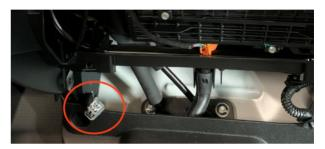
5. Route the pin end of the speed/reverse wires from the main dash aperture through and down toward the fuse panel. The bare ended wires will remain in the dashboard aperature for use on the new head unit.
