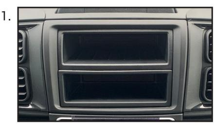
Begin by using a panel removal too to unclip the two pockets that sit where the main head unit would normally sit.
