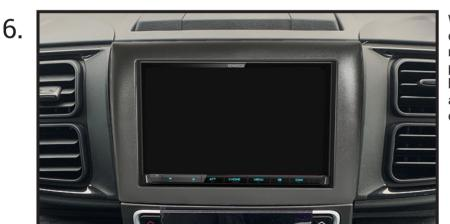
With the cage in place, and the head unit connected correctly, proceed to slot the radio into the dashboard until it clips into place. Carry on to finish the installation by placing the trim around the head unit and re-assembling the dashboard in revere order.
