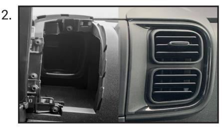
Use the panel removal tool to unclip the entirety of the side air vents. Once free, simply pull them out of the dashboard and set them to one side.
