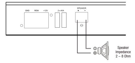
Please note that this unit is a mono block amplifier and has only one channel. Connecting to either the positive or negative of either of the two connections will end in the same result as both positive connections (or both negative connections) are tied together inside the unit. For example, if you connect two 4 ohm subwoofers, the amp will parallel the connections for a 2 ohm load.
