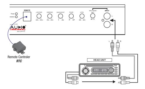
The **SERIES** amplifier offers RCA-Inputs, which are connected through cinch cables with the preamplifier-outputs of the head unit. **IHLAC** and **RCA IHI** adapter cable can be purchased as accessories if the head unit has no RCA output. The **IHI/LOW** button must be switched to "**IHI"**. If the **SERIES** amplifier gets a signal from head unit output, the amplifier will turn on.
