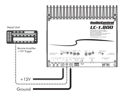
In this example, the head unit has a +12V trigger output that is connected to the LC-1.800 remote input terminal. When the head unit is turned on, it will turn on the LC-1.800 amplifier.
